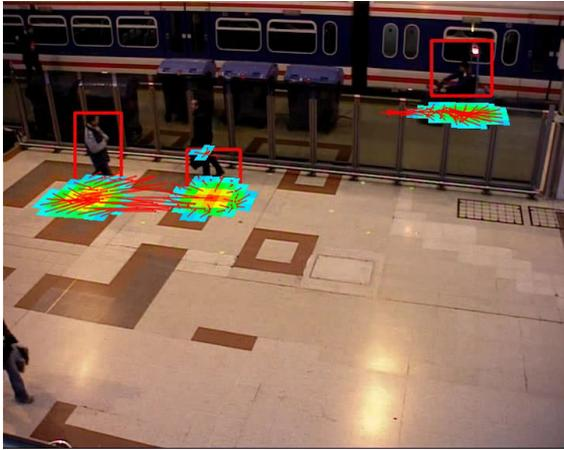
Figure 2 – Example of BOF output using a computer vision pedestrian detector as input (red boxes). The BOF output is projected back on the image. It represents a grid of occupancy probability (blue-to-red mapped color) and the mean velocity (red arrows) estimates.
